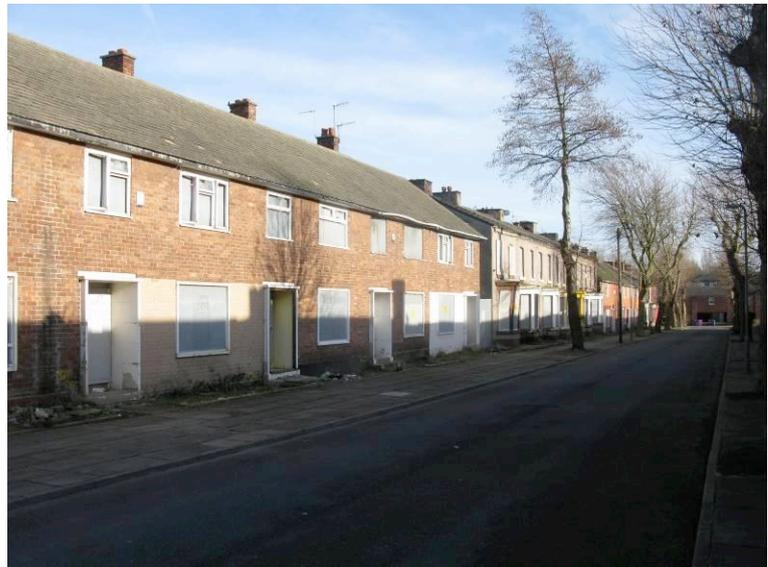
Inevitably with such buildings in long terraces and over a relatively wide area, there are some areas of local movement. These tend to be through window openings, typically bays. Elsewhere there is some bowing of the front elevation concentrated a short way above ground level. However I would stress that related to the in excess of 400 buildings only a few of the buildings are affected significantly and to an extent that would warrant significant intervention or local re-building.
